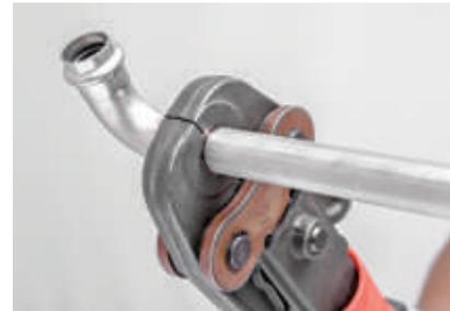
**Press joint:** Initiate the pressing procedure by pressing the start button for approximately 3 seconds. The pressing procedure will run automatically and should not be interrupted prematurely. This ensures a permanent joint that is sealed and has the required tensional and axial force locking properties. After completing the pressing process, the pressing tool can be removed from the pressed connection by opening the press jaw.
